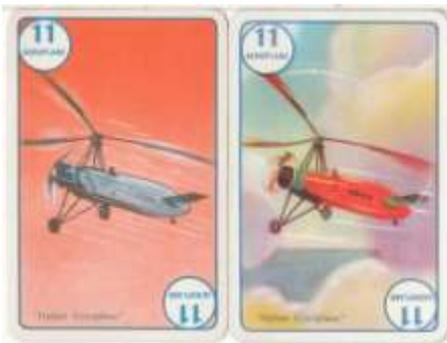
**Aeroplane No 11** The Hafner AR III Gyroplane was an experimental autogyro built by Martin-Baker in the mid 1930's. It was demonstrated to the Royal Aircraft Establishment in 1937 and leased to them for trials. Unusually it featured a rotor system with adjustable pitch blades which were to become a feature of all future helicopters. The motive power was provided by a 90 hp radial piston engine. No production of the machine ever came about however and the prototype was scrapped after the war.
