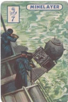
Most of the Royal Navy Mine Laying ships were small vessels of around 120 ft length. Many were built as Merchant vessels originally and were commandeered and converted by the Royal Navy. The illustration on this card seems to show an early type of mine being laid. It would be secured to the bottom on a line which left it just below the surface. The mine exploded on contact with any vessel.
